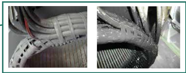
Grey treatment (marinization) on the left, TOTAL treatment shown on the right.
